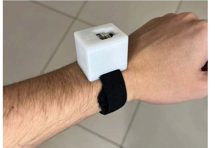
Fig. 5. Smartband worn on the wrist during operation.
