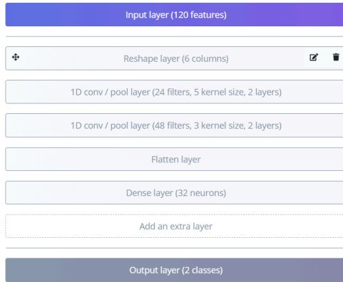
Fig. 7. 1D CNN architecture deployed on the M5Stack AtomS3R-Ext comprising an input layer (120 features), a reshape layer, two 1D convolution/pooling blocks, a flatten layer, a dense layer (32 neurons), and 2-class output layer.
