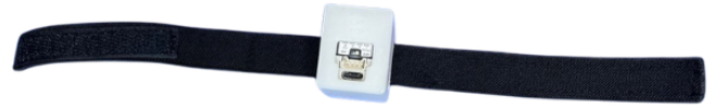
Fig. 4. Prototype of the wrist-worn smartband: M5Stack AtomS3R-Ext enclosed in a 3D-printed PLA case and fixed to the wrist via a Velcro strap.
